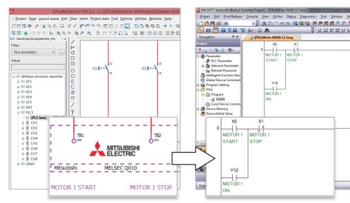
Exchange of EPLAN function text with iQ works label
